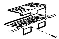
4. Remove and save the screw that holds blower motor to microwave.
